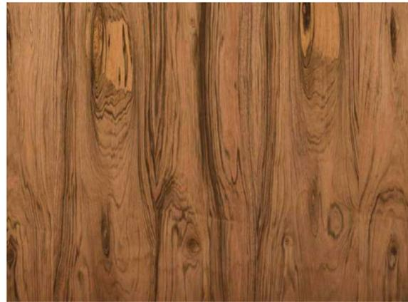
A tangent cut across the growth rings is what produces a crown cut veneer with a pattern that is characterized by straight grain intermixed with crowns that represent cathedral arcs.
